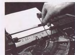
To type a character not included on the duclos keyboard an auxiliary type bar from the special case (above left) and attach it to the auxiliary setting device above the carriage (above) and it is transferred to a vertical position in front of the other type bars ready to be struck (below)
